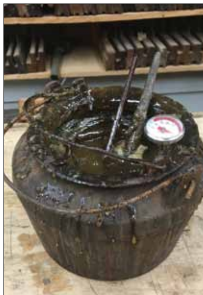
A glue pot, with brushes and a thermometer
